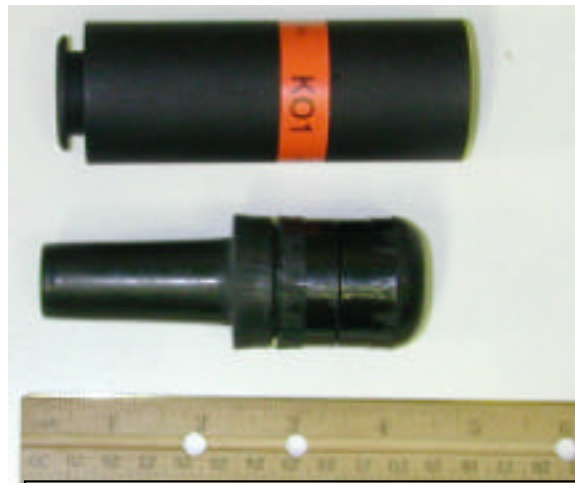
Photo #3 Sage Control Ordnance, Inc. KO 1 Cartridge & Plastic Baton Round
